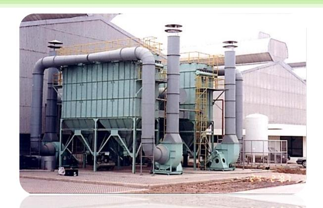
Bag filter dust collector shaking type and pulse jet type with casing of carbon steel or stainless steel and size from 4 bags up to 1,000 bags. We not only sale to end user but also supply to other dust control companies.
